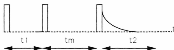
Fig. 4. Pulse sequence used for two-dimensional exchange NMR spectroscopy.
